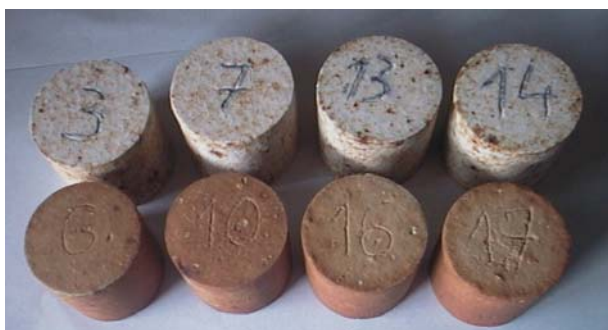
Fig. 5. Specimens treated at 1635°C (3+7-"SN"; 13+14-"SM"; 6+10-"BN"; 16+17-"BM")
