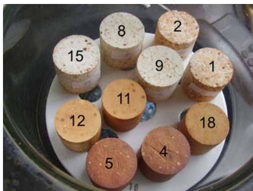
Fig. 3. Specimens treated at 1580 and 1700°C 1+2-"SN" at 1700°C; 8+9-"SN" at 1580°C; 15-"SM" at 1580°C; 4+5-"BN" at 1700°C; 11+12-"BN" at 1580°C; 18-"BM" at 1580°C)
