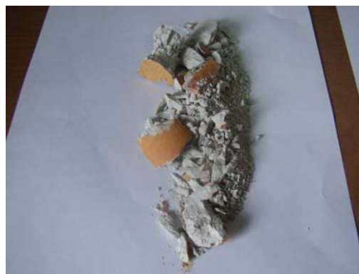
Fig. 4. Destroyed "BM" at 1580°C
