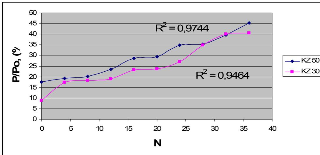
Fig. 1. Damaged surface level ( $P/P_0$ ) versus number of quench experiments (N)
