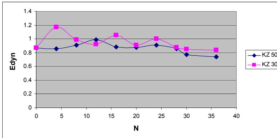
Fig. 2. Dynamic Young modulus of elasticity versus number of quench experiments (N)
